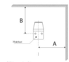
The distance from wall (A) is more than 34 cm. The distance from ceiling (B) is more than 48 cm.
