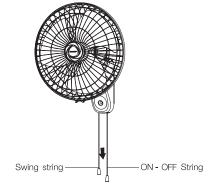
Pull swing string to let the electric fan swing left right and pull this string once again when you would like the electric fan to stop swing.
