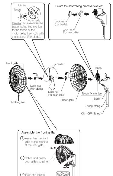
If the arilles and blade are not tightly assembled, the unit will be shaking.
